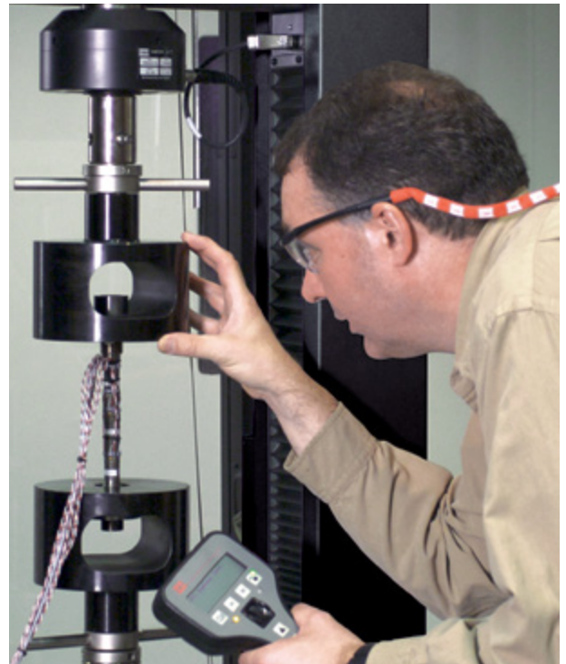
Load Frame Alignment
